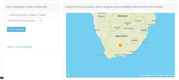
The "Check Coverage" section of the website allows you to check if a certain area has Sigfox capability. To use the coverage map, simply get the coordinates of the area you'd like to check and copy that into the first textbox, and select the correct Sigfox network according to country.
